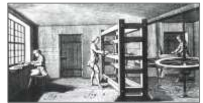
Diamond cutting in the 18th Century. The first worker rubbed two diamonds against each other, the second sprinkled the polishing wheel with diamond powder soaked in oil, and the third turned the wheel of the scaif.
