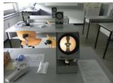
The proportion scope provides percentages based on the proportions and the symmetry of certain characteristics of round brilliant cut and modified brilliant cut diamonds.
